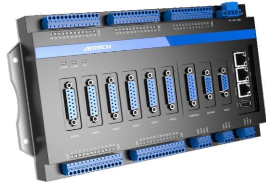
AMC1600P SUPPORT 6 AXIS 36 INPUT 30 OUTPUT
