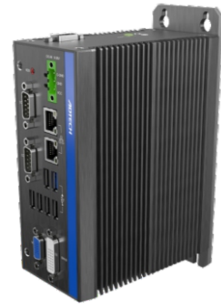
AMC3000E IEC61131-3 programming can support 32 axis Bus
