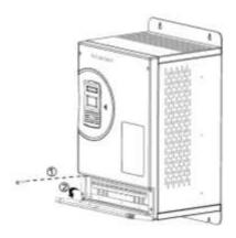
Figure 3-7 Open wiring cap
